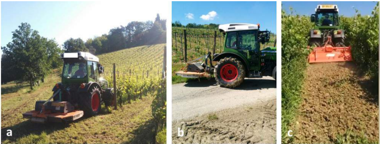
Figure 2: a,b) mower c) soil incorporation with rotary tiller
